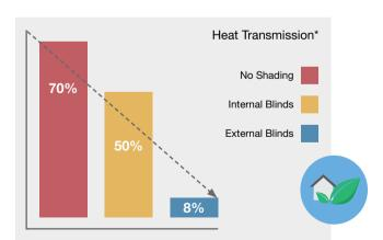
Blocking upto 92%\* of the suns near infra-red heat rays, our external blinds can reduce interior room temperatures by more than 10 degrees centigrade, which in turn can reduce the energy consumption otherwise needed to cool down a hot room by more than 80%.
